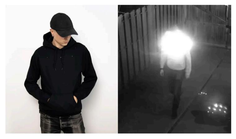
Although unnoticeable to human eyes, the garment s infrared additions wreak havoc on surveillance cameras that utilize the light spectrum to see in evening darkness. Emitting the flashing infrared bursts from the hoodie will force nearby cameras auto exposure to try correcting for the brightness, thus obscuring a wearers face in a bright, pulsating light.
