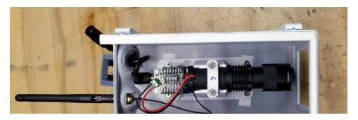
Internally, each camera has an off-the-shelf LED flashlight that's had its power button rigged up to an ESP8266. Once they've been manually pointed to the appropriate spot on the wall, [Mac] can turn each camera's spotlight on and off over WiFi. Rather than rely on the gallery's infrastructure, all of the cameras connect to the ESP32 M5Stack that serves as the central controller via ESP-Now.
